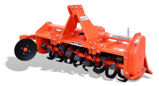
Vivo is Specially designed for soft and loose soil. Its light weight technology makes it perfect for puddling in paddy fields. The helical-shaped rotor on the Rotary Tillers decreases horsepower required to drive units. They are designed so they enter the field at different times for more efficiency. These are sized right for subcompact tractors and are designed to till soil for seedbed preparation.
